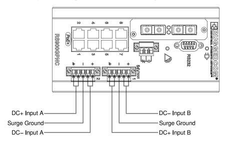
Figure 2.5. DC Power Supply Wiring and Grounding
